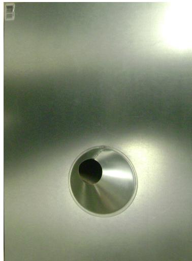
PIPE FLASHINGS ARE MADE OF 26 GAUGE GALVANIZED STEEL, ASTM A-653. THEY HAVE LOCK-FORMED BASES. TYPICAL INSTALLATIONS OF STEEP-PITCH PIPE FLASHINGS ARE ON ROOFS WITH SLOPES RANGING FROM 6/12 TO 12/12 PITCHES.
